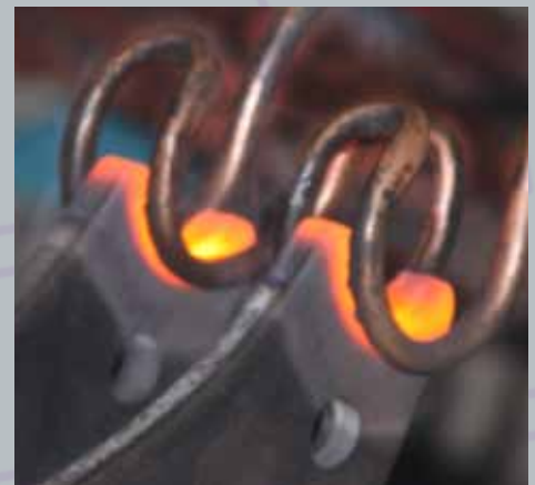
Both cam and anchor ends are heat-treated to more than 1,000° F to prevent disfiguring and loss of brake geometry. This extends brake life and improves braking performance.
