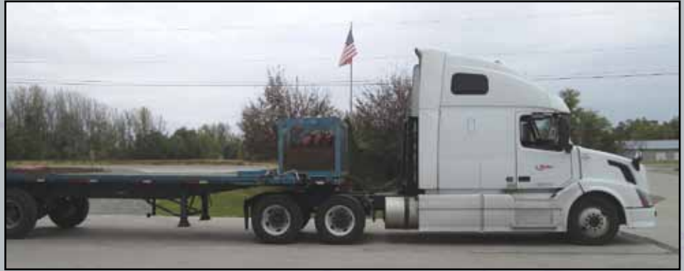
New Reduced Stop Distance (RSD) regulations require three axle tractors to stop in 250 ft or less when laden with a trailer (pictured above), and 235 ft or less for tractors unladen (not pulling a trailer).
